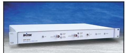
The MSP-220-C provides a state-of-the-art solution for video switching centers. It is used in operations that require conversion of analog video with multiplexed audio signals to video with separate audio channels. Full bi-directional operation is supported through the use of one modulator and one demodulator circuit in the same 1 RU unit.
